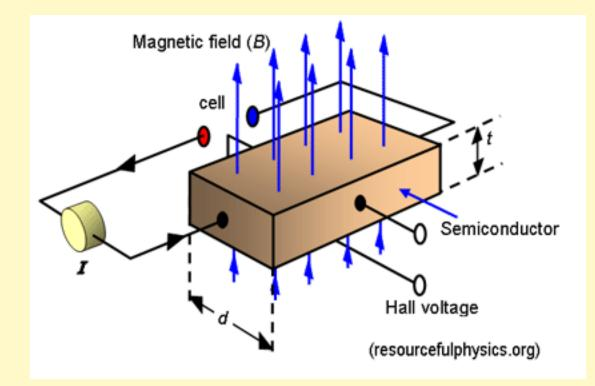
Hall voltage is produced by charge accumulation on sidewalls
