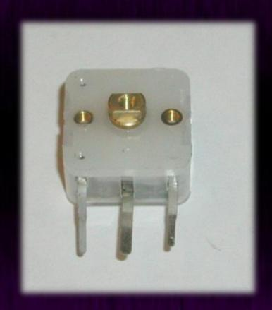
A capacitor whose capacitance can be varied. These are usually made up of one or more moving plates and one or more non moving plates separated by the dielectric. By moving the plates, we can vary the capacitance. And it is used in a radio tuner.
