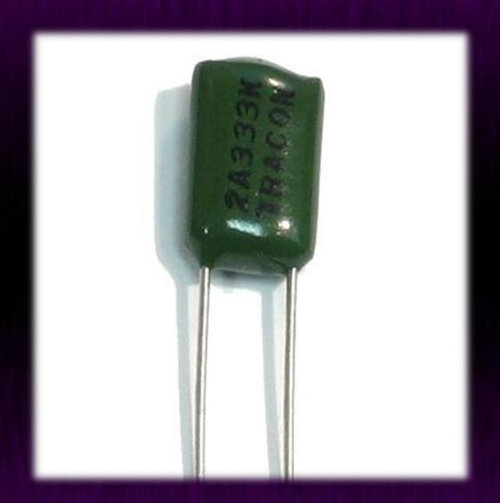
Type of capacitor that can be connected any way in a circuit. There is no positive or negative. Common types of non-polar capacitors are ceramic, mica and some electrolytic.
