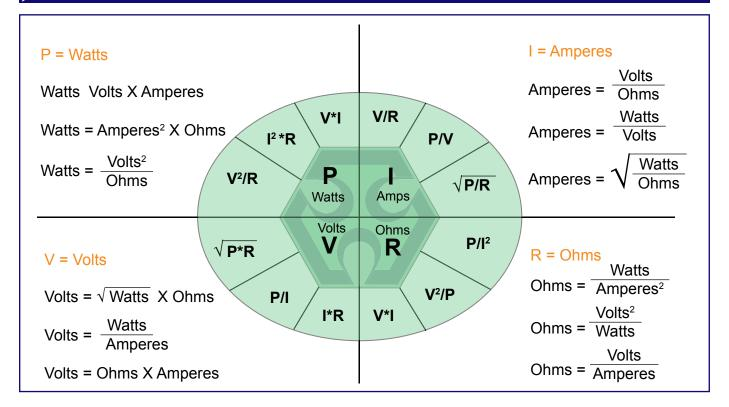
Ohm's law is a simple equation that shows the relationship between resistance, voltage and current through a metal wire, or some other type of resistive material. In mathematical terms, Ohm's law is written as:
