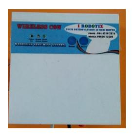
Motor Con is an intelligent electronic device connected to your motor starter to let you remotely control and protect your three phase pump set from anywhere in the world through the motor Con App, or an SMS, or a phone call or a missed call, making use of GSM network for global connectivity
