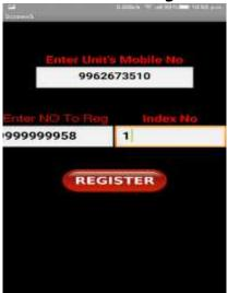
Up to 10 user number we can able to register, first number is the master number Enter Units Mobile No-98######(GSM SIM NUMBER)
